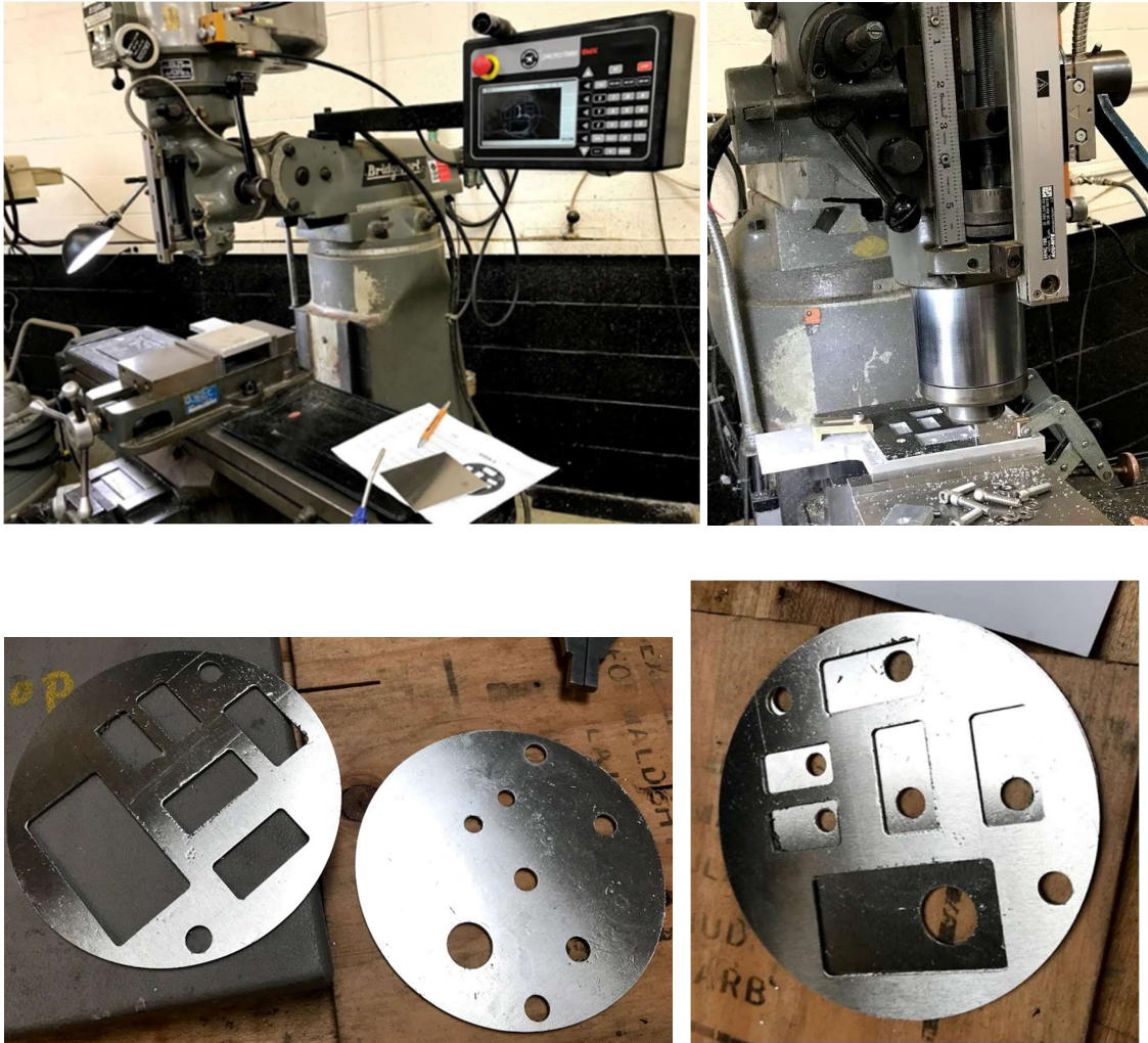
Figure 5-6 Mask Fabrication clockwise from top : (a) ProtoTRAK SMX Milling Station (b) Sheet Mask being cut (c) Finished mask set (d) Finished Mask Set overlaid
