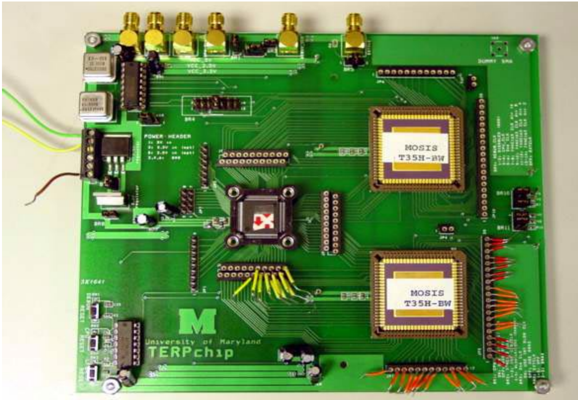
Figure 9: Printed circuit board containing our fabricated processor and safe storage integrated circuits, along with miscellaneous support circuitry.
