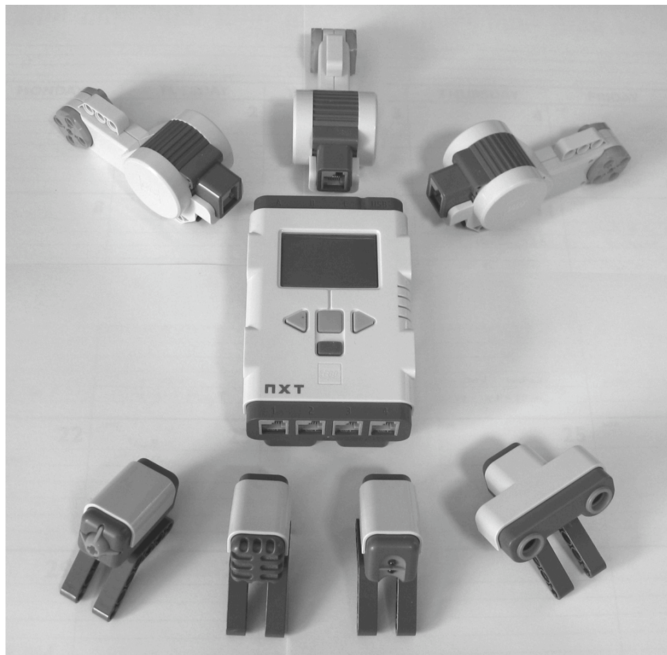
Fig. 6.13 Sensors and motors arranged around the NXT controller.
