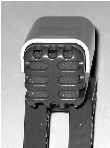
Fig. 6.8 The LEGO touch sensor (a contact switch) is a passive device that does not require power to function.
