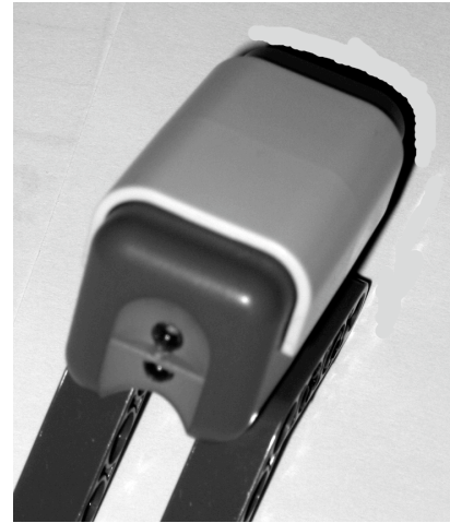
Fig. 6.10 The LEGO light sensor is an active device that requires power to light its IR source. Its readings range from 1 (dark) to 100 (bright).
